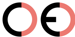
False CE Mark (too far)
